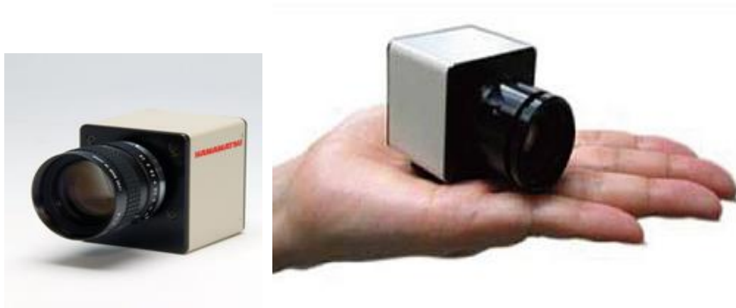
Figure 3. Intelligent vision sensor with a camera that performs high-speed parallel image processing by using the number of parallel processing elements equal to the number of pixels. The camera processing mode can be changed by the program. For example, data acquired with multiple cameras (1 to 4 cameras) can be synchronously fed to the parallel processing circuit that performs real-time processing to output only the calculated results or control signals. This allows real-time control of images containing a vast amount of information with low latency (lag).
